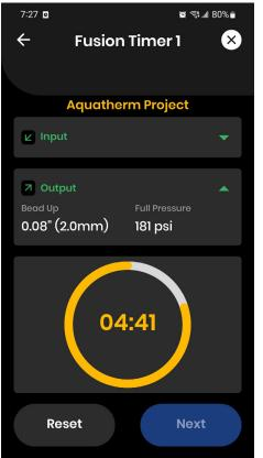
Once you've finished selecting the pipe size, pipe SDR, fusion tool manufacturer, specific tool, and input the drag pressure and ambient temperature, you'll be able to start your heating timer, followed by the cooling timer.
