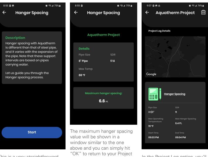
This is a very straightforward tool to use. Simply start the guide, input values for pipe size, pipe SDR, and maximum operating temperature.
