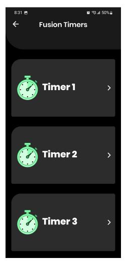
We encourage installers using Aquatherm to run multiple fusions at once. As such, we have allowed for the installer to run three simultaneous timers. Heating & Cooling Timers
